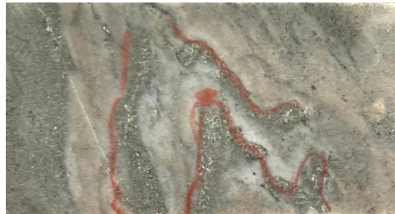
Buckling of mineralized B Type porphyry vein
